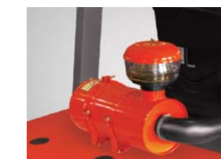
Pre-cleaner engine air intake
